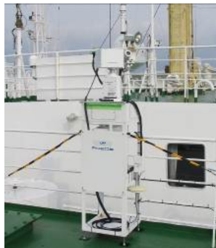
Figure 1. Solar tracker and telescope. The sunlight collected into optical fiber was introduced into the OSA that was installed in an observation room in the MIRAI.
