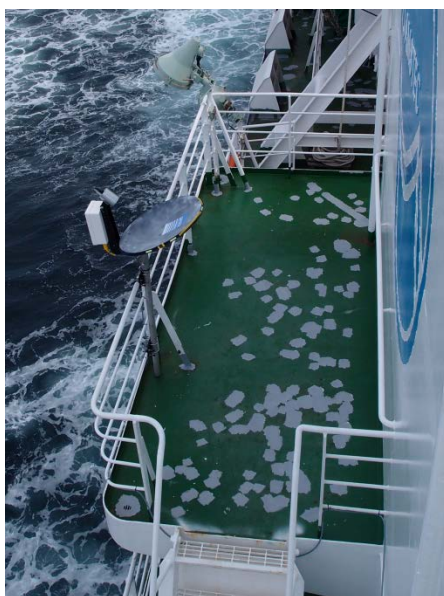
Fig. 2.8-2: The micro rain radar, installed on the starboard side of the anti-rolling tank.
